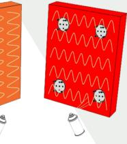
Spray wall and surface of PanelHush panel with Gluehush contact spray adhesive, ensuring that 100% of both surfaces are covered.
